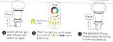
⚠ If the light not blink slowly, the linking failed. Pls switch off the light again, and follow the above steps again.
